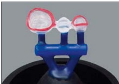
As is customary in casting / press procedures, the mould is fitted with wax sprues and waxed onto the funnel former. When doing so, the instructions provided by the alloy manufacturer and press-ceramic manufacturer must be observed.
