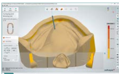
10 Block out lower jaw undercuts.
