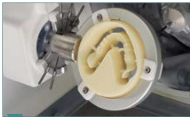
4 Mill the wax disc for the full-sized wax try-in (mandible).
