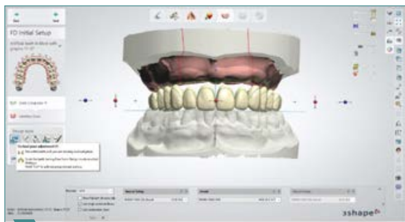
5 Selection of tooth library and rough positioning of the tooth setup.
