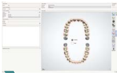
2 Create denture gingiva; Type: VITA VIONIC BASE with artificial teeth; Material: VITA VIONIC BASE HI; Manufacturing Process: Milling VITA VIONIC BASE.
