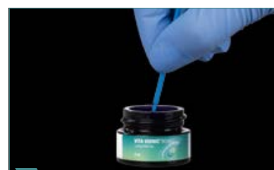
3 Mix the two components for 30 seconds to prevent air bubbles.
