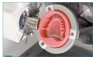
3 Mill the wax disc (UJ and LJ) for the try-in.
