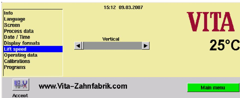
Adjust the lift speed with the slide control.
