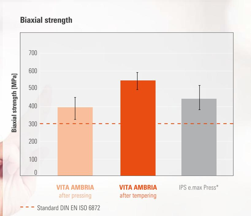
Source: Internal study, VITA R&D, Measurement of biaxial strength of abovementioned materials in accordance with ISO 6872 (with modified sample geometry), (Gödiker, 1/2019, [1] see back of prospectus)
