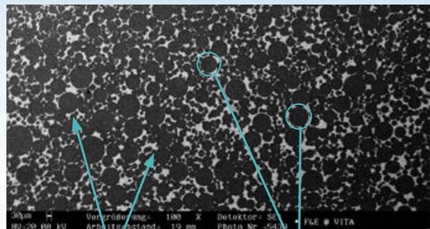
Matrix with polymerized SiO<sub>2</sub>
