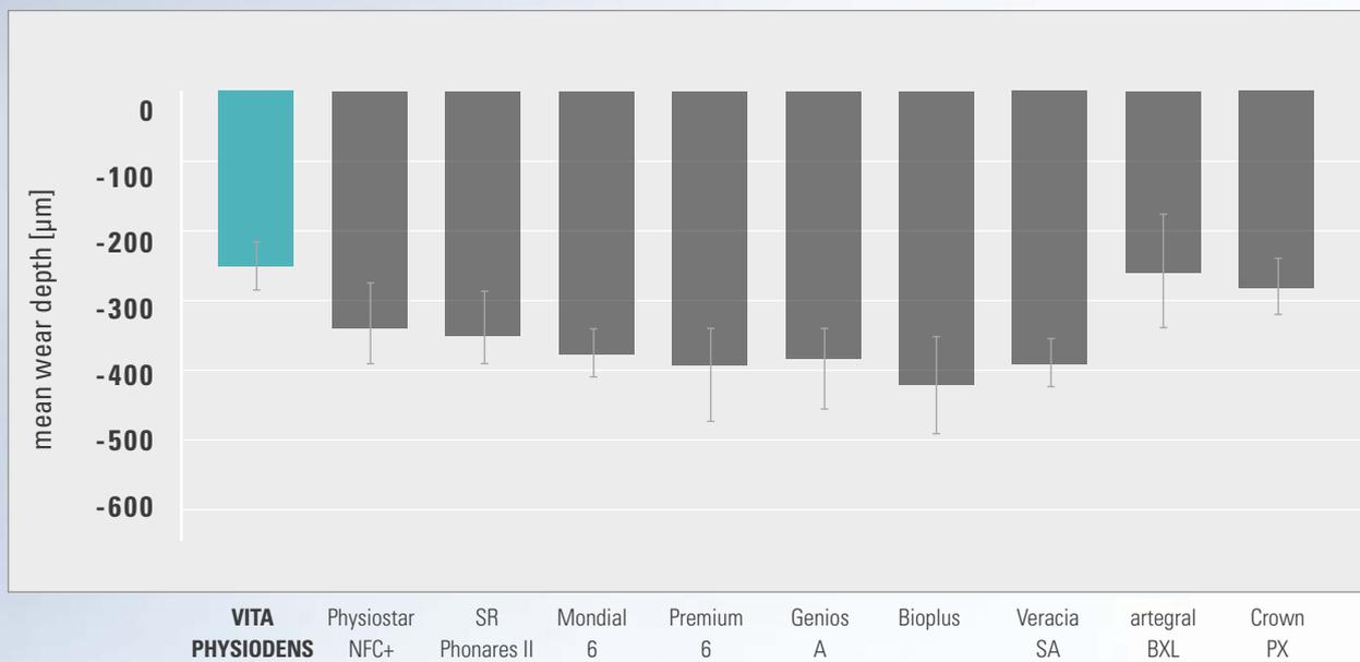
**Graphic:** Average depth of the signs of wear of the abovementioned tooth lines after pin-on-block wear test in the chewing simulator with steatite balls as antagonist and eight test samples each per line.
