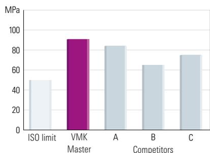
Fig.: 3-point flexural strength according to ISO 6872
