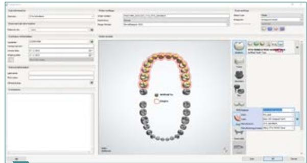
2 Crear la encía: Type: Base with designed teeth; Material: VITA VIONIC BASE HI; Manufacturing Process: Milling VITA VIONIC BASE.
