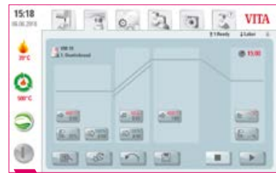
3 Firing window with single-stage curve.
