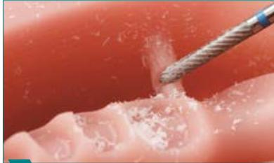
**4** Separate the denture bases from the disc.
