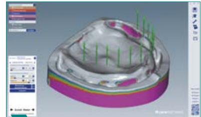
**6** Design the base surface of the maxilla prosthesis (blocking the model out).
