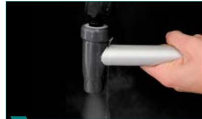
6 Clean the tooth blanks and remove any residual wax.
