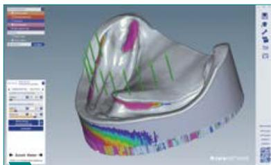
**7** Design the base surface of the mandible prosthesis (blocking the model out).
