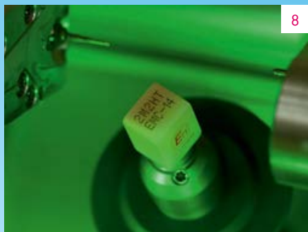
Fig. 8 The highly translucent, hybrid ceramic block in the color 2M2 clamped in the grinding machine.
