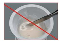
Streaks and bubbles can be avoided by observing the correct mixing ratio and by evenly mixing using the instrument along the base of the mixing container.
