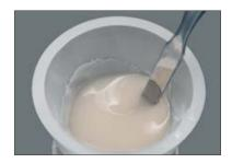
Once the material has been mixed evenly, it has a doughy consistency and can be processed following an appropriate expansion time (approx. one minute). The processing range is approx. four to five minutes, depending on the room temperature.
