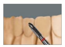
Finishing and corrections to the shape are carried out using carbide milling tools at a speed of 15,000 rpm.
