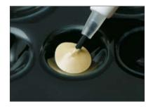
⚠ **Note:** Turn back the syringe of the light-sensitive OPAQUE PASTE by at least one turn after dispensing some material and seal it again immediately.
