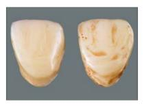
Photo 1: to the left: completely polymerized, hardly any discoloration to the right: incompletely polymerized; strong discolorations
