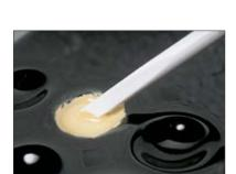
First add the liquid into the depression of a black ceramic mixing plate. Then add the powder and stir with a plastic spatula for approx. 30 sec. to obtain a homogeneous, thin mixture. Mixing ratio: five drops of liquid and one measuring spoon of powder (to obtain approx. four units). Mixing ratio: five drops of liquid and one measuring spoon of powder (to obtain approx. four units). The use of a metal spatula is not recommended, since it may result in color changes.
