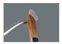
The metal framework is cleaned after sandblasting. Use only dry compressed air (with water separator) or a clean dry brush for cleaning.
