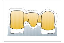
Use BASE DENTINE to model the copings and the pontic in reduced tooth size. The approximal connections must have a diameter of at least 3.5 mm (10 mm²).
