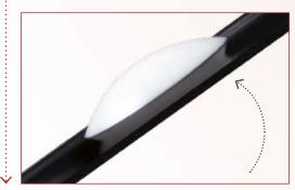
2. Testing of stability by tilting the plate
