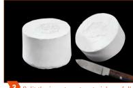
3 Split the investment material carefully using a knife on the predetermined breaking point.
