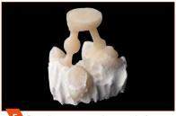
Fine divestment and removal of reaction layer with abrasive glass beads at a pressure of 2 bars.
