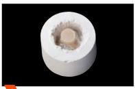
Perform rough divestment with Al<sub>2</sub>O<sub>3</sub> (50 μm grain size) at a pressure of 4 bar.
