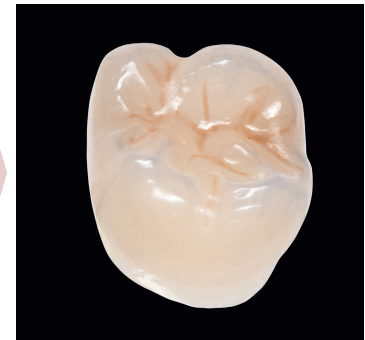
Stained VITA ENAMIC crown after wear test
