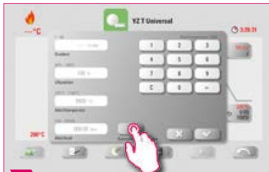
5 Select second cooling phase: "Controlled cooling."
