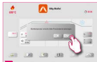
3 Once you have inserted the pressing material, confirm the message. The lift plate will move into the firing chamber.
