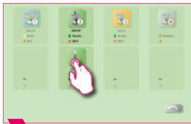
2 Multifurnace: Press and hold the firing program button to move it if you want to use another firing device.
