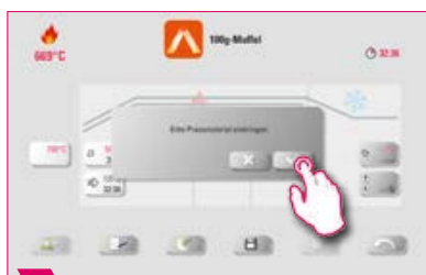
2 Confirm the message. This causes the lift plate to move to the bottom position.
