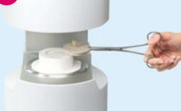
Remove the firing tray and restoration
