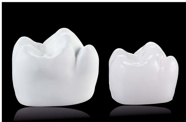
Figure 6: Example of sintering shrinkage of zirconia by approx. 20 %
