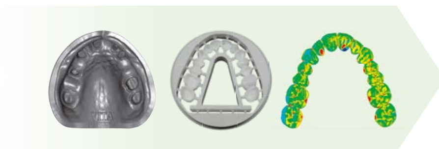
Figure 14a/b/c: a) model; b) milled, multi-unit VITA YZ structure; c) wrap software with overlapping structures (from left to right)
