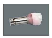
Use wax or silicone to protect or to seal the emergence profile and the screw channel of the zirconia abutment. Protect connection geometry with a model analog or polishing cap [3]\*.
