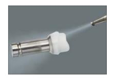
Then clean in the ultrasonic bath or with alcohol or steam and dry with oil-free air.
