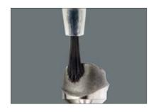
The surface to be bonded must not be touched after cleaning to avoid any contamination, which may have a negative effect on the adhesive bond.
