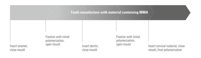
Figure 12: Schematic illustration of manufacturing procedure of (P)MMA denture teeth; source VITA R&D
