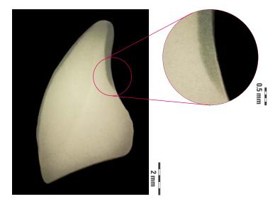
Figure 11b: Light microscope image of the sectional view of a VITA denture tooth made from MRP composite (VITAPAN EXCELL®); source VITA R&D
