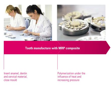
Figure 11a: Schematic representation of the manufacturing procedure of denture teeth made from MRP composite; source VITA R&D
