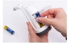
Figure 4 - Changing batteries: Remove battery on left
