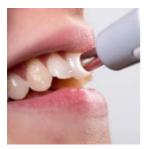
While holding the measuring tip against the central dentin part of the tooth, press the measurement button. Hold the measuring tip against the tooth until two short consecutive signal tones mark the end of the measurement process. The VITA Easyshade LITE displays the measurement results.
