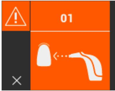
If you lift the measuring tip off the tooth before the instrument produces a signal tone, an error message or faulty measurement will be displayed and you will have to perform the measurement again.
