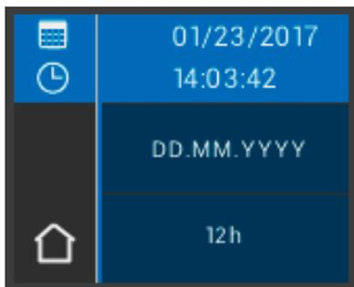
Pressing the date field in Settings allows the user to switch the type of display between DD.MM.YYYY and YYYY.MM.DD, as well as between the 12 and 24 hour display.
