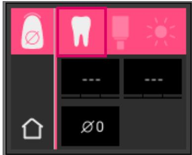
With averaged shade determination, up to 30 measurements can be performed on a natural tooth. The determined tooth shade is displayed in the VITA SYSTEM 3D-MASTER and VITA classical A1–D4 tooth shade systems.
