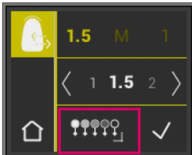
To select interpolated shades, please switch over to the extended mode by using the
