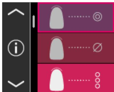
To determine the base shade of a natural tooth, touch the symbol for base shade determination in the main menu. Trigger the measurement by pressing the measurement button and place the measuring tip flush in the central area of the dentin of the tooth. The measurement is performed without further interaction as soon as the instrument is stable on the surface of the tooth. Once the measurement is completed, the VITA Easyshade V produces an acoustic signal.
