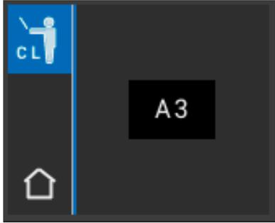
To measure, place the measuring tip flush with light pressure in the upper third (below the neck of the tooth) of the shade tab. Now press the measurement button. The closest tooth shade is displayed.
