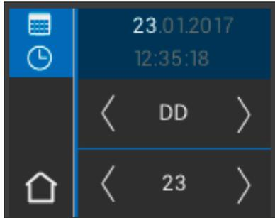
Touch the top button, which displays date and time. Use the arrows to scroll to the right or left in order to set the date and time.
