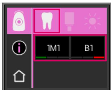
To display the measured tooth shade, select the tooth symbol in the top bar. The measurement result is displayed in the VITA SYSTEM 3D-MASTER and VITA classical A1–D4 tooth shade systems. All 29 VITA SYSTEM 3D-MASTER and all 16 VITA classical A1–D4 shades can be measured.
