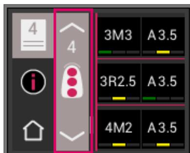
After selecting the VITA classical A1–D4 or VITA SYSTEM 3D-MASTER shade specification, you will return to the detail display (Fig. shows details of the VITA SYSTEM 3D-MASTER shade specification) as described in 6.1.3 and 6.1.5.
