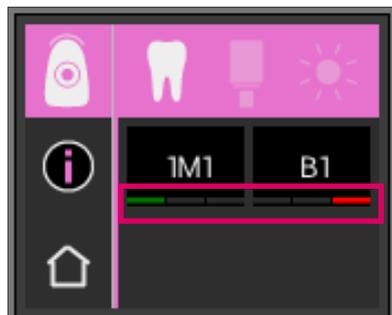
Using a traffic light function, the VITA Easyshade V shows you how close the measured tooth shade is to the next VITA SYSTEM 3D-MASTER or VITA classical A1–D4 shade. The degree of the match is indicated by a green, yellow or red bar.
