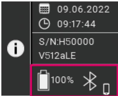
If the Bluetooth icon is white, Bluetooth is activated, but not yet paired with a device. The icon beside the Bluetooth icon indicates the selected connection mode (Windows PC or mobile device). More information on the connection modes is provided in section 9.
