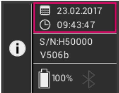
When you tap "Date and Time" in the upper section, you are taken directly to the settings, where you can make changes to the date and time. The serial number and the software version are displayed in the middle area.
