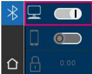
Go to the Bluetooth settings. Move the upper Bluetooth slider for a Windows PC to the right to activate Bluetooth. The padlock icon is unlocked automatically, making VITA Easyshade V visible for two minutes. If the padlock (icon) is locked, you can touch it to make VITA Easyshade V visible again.
