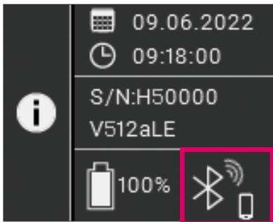
If the VITA Easyshade V is paired with a device, radio waves are displayed on the top right next to the Bluetooth icon. To the right of the Bluetooth icon, you can see if it is paired with a Windows PC or a mobile device. You can tap the Bluetooth icon to go directly to the Bluetooth settings and make changes there. See section 9.
