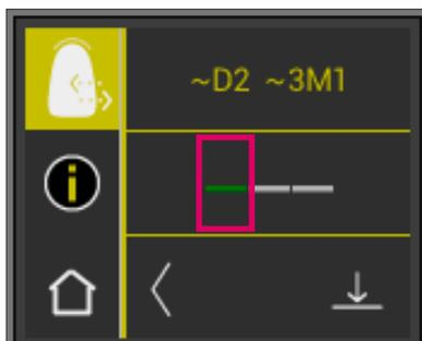
**GREEN** means "Good." This means that there is little or no difference between the base shade of the restoration and the target shade that it was compared to. To obtain extended shade information, please touch the traffic light symbol in the middle of the display.
