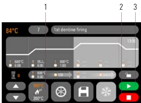
Figure 4 – Starting/switching to standby
