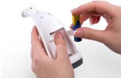
Figure 5 – Changing batteries: Insert new battery
