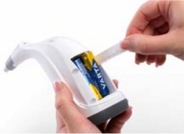
Figure 3 – Changing batteries: Remove battery on right
