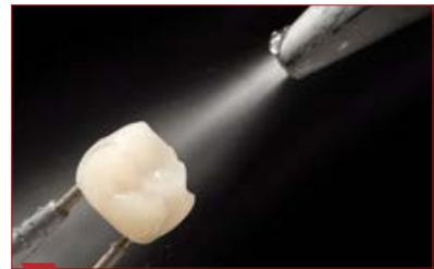
**3** Clean the surface carefully (e.g., using a steam jet).
