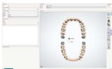
2 Denture Gingiva anlegen: Type: VITA VIONIC BASE with artificial teeth; Material: VITA VIONIC BASE HI; Manufacturing Process: Milling VITA VIONIC BASE.
