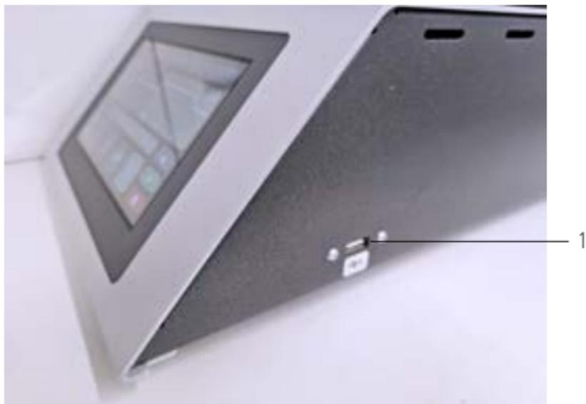
*Figure 1 – Inserting the VITA USB WiFi modem*
