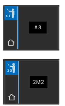
To measure, place the measuring tip flush with light pressure in the upper third (below the neck of the tooth) of the shade tab. Now press the measurement button. The closest tooth shade is displayed.
