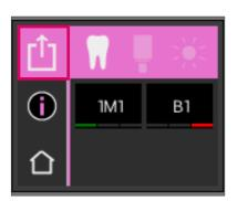
Perform a measurement with the VITA Easyshade V. To transmit the results, touch the measurement results icon at the top left. The results can be transmitted from all measurement modes and from the measurement memory by touching the corresponding icon at the top left. Restoration mode results cannot be transmitted.
