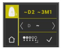
All subsequent shade measurements in this mode (without saving) are compared to the user standard, and the degree of match is displayed in red, yellow or green with the LCh value deviations.
