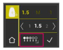
To select interpolated shades, please switch over to the extended mode by using the **PPPPPP** button.
