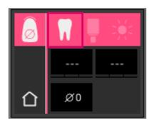
With averaged shade determination, up to 30 measurements can be performed on a natural tooth. The determined tooth shade is displayed in the VITA SYSTEM 3D-MASTER and VITA classical A1–D4 tooth shade systems. It is recommended that at least four measurements are taken. To do this, the measuring tip is shifted slightly on the tooth after each measurement and when a new measurement is taken.
