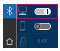
Go to the Bluetooth settings. Move the upper Bluetooth slider for a Windows PC to the right to activate Bluetooth. The padlock icon is unlocked automatically, making VITA Easyshade V visible for two minutes. If the padlock (icon) is locked, you can touch it to make VITA Easyshade V visible again.
