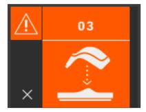
If there is only a single signal tone, the white balance could not be correctly performed. In this case, an error message appears on the display. Acknowledge the error message by touching the x-symbol on the display and repeat the white balance.
