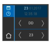
Touch the top button, which displays date and time. Use the arrows to scroll to the right or left in order to set the date and time.
