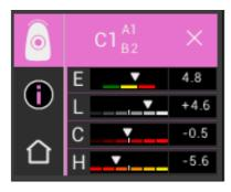
This illustration shows the shade differences between the measured tooth shade and the closest VITA classical A1–D4 shade. The bars represent the shade deviations graphically.
