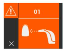
If you lift the measuring tip off the tooth before the instrument produces a signal tone, an error message or faulty measurement will be displayed and you will have to perform the measurement again.
