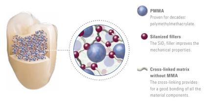
Schematic structure of MRP composite; Source VITA R&D
