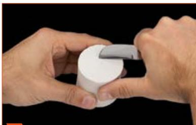
**2** Break the edges of the investment ring without allowing investment material to fall into the channel.
