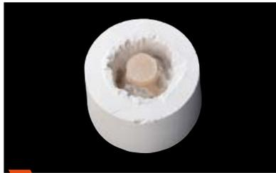
**4** Perform rough divestment with  $Al_2O_3$  (50  $\mu m$  grain size) at a pressure of 4 bar.
