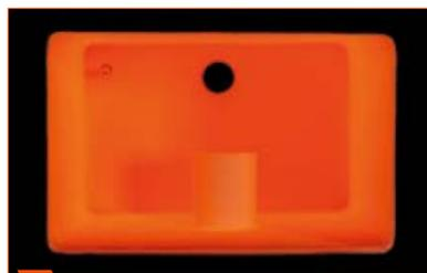
**3** Place the investment ring in the furnace with the opening facing down. No contact with the furnace wall.
