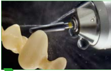
1 Processing with turbines under water cooling.
