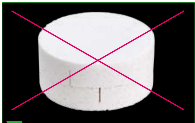
10 Do not lay one sintering dish directly on top of the other.
