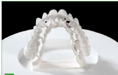
5 Separated and reworked restoration with sintering support.
