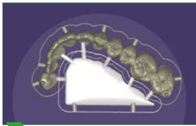
1 Sintering tongue and sintering drops
