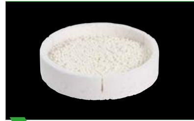
3 Fill the sintering dish MS with sintering pearls (a pearl bed of at least three layers).
