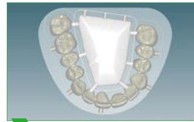
3 Sintering tongue before skeletonization
