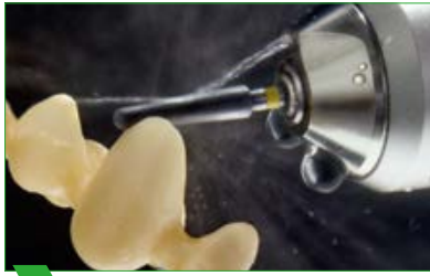
1 Processing with turbines under water cooling.
