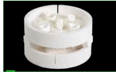
6 Stack sintering of color/multicolor restorations.
