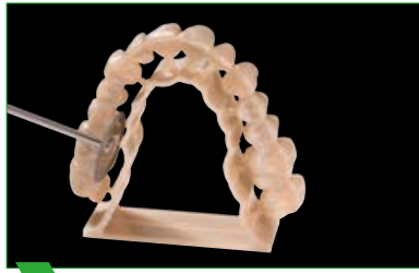
2 Carefully separate the bridge construction.
