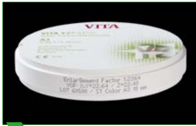
1 Enlargement factor as plain text on disc
