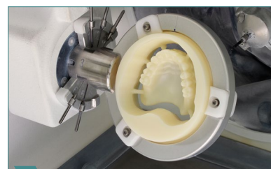
3 Mill the wax disc for the full-sized wax try-in (here: UJ).
