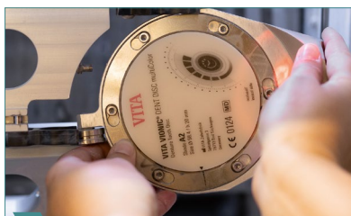
4 Clamp the VITA VIONIC DENT DISC multiColor into the holder of the milling machine. Mill dental arch/tooth elements.
