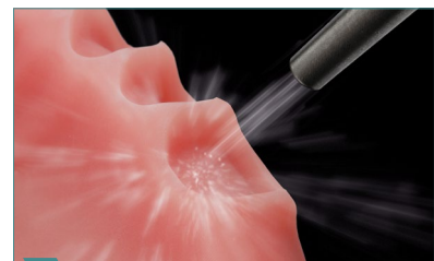
6 Sandblast the milled cavities of the denture bases.
