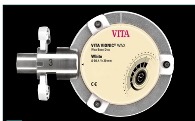
2 Clamp the white wax disc in the holder system.
