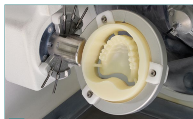
3 Mill the wax disc for the full-sized wax try-in (maxilla).
