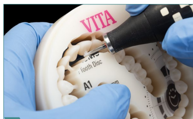
5 Cut out the dental arch/tooth element from the disc using crosscut carbide cutters.
