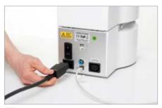
2 Connect the firing unit to the power supply.
