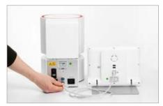
1 Connect the firing unit and control unit using the connection cable.
