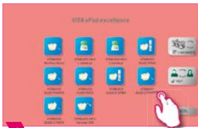
1 Press on the desktop and hold until the desktop editing menu is activated.
