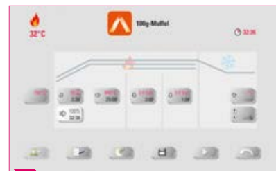
3 Briefly press firing program to go to the firing window.
