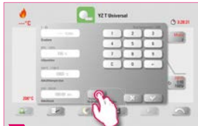
5 Select second cooling phase: "Controlled cooling."
