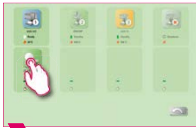
2 Multifurnace: Press the firing program and hold and move if you want to use another firing device.
