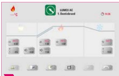
4 Firing window with single-stage curve.
