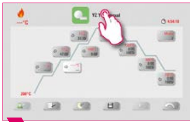
1 Select firing chamber temperature / holding time.
