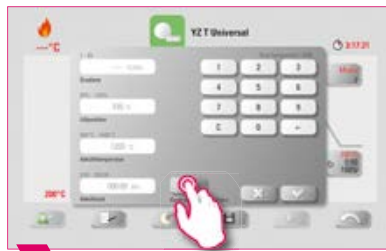
2 Select first cooling phase: "Controlled cooling."
