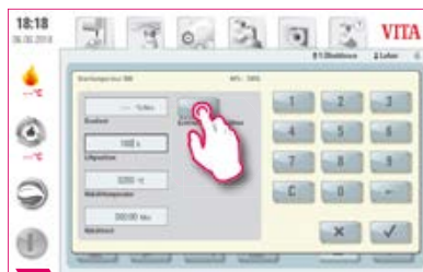
8 Select third cooling phase: "Controlled cooling."
