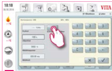
5 Select second cooling phase: "Controlled cooling."
