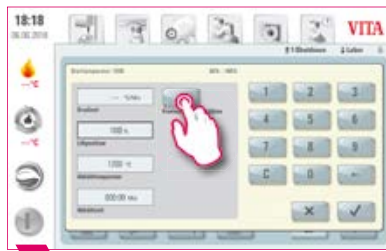
2 Select first cooling phase: "Controlled cooling."
