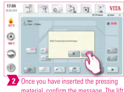
2 Confirm the message. This causes the lift plate to move to the bottom position.
