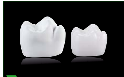
3 Molar before and after sintering; sintering shrinkage of about 20 percent
