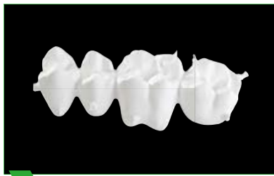
1 Milled restorations immediately after the CAM process.
