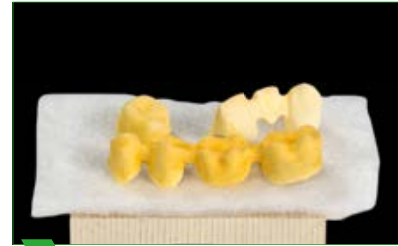
6 Dry the restorations thoroughly before sintering.
