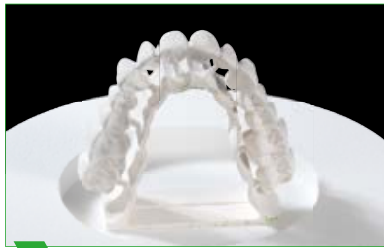
5 Separated and reworked restoration with sintering support.
