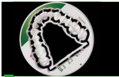
1 Bridges with skeletonized sinter support following the milling process.
