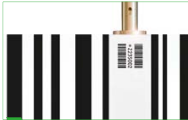
2 Enlargement factor as barcode on block
