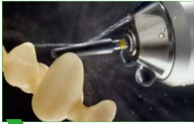
1 Processing with turbines under water cooling.
