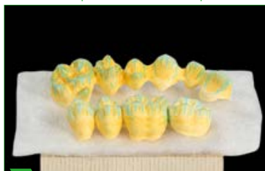
11 Restoration on firing tray, ready for pre-drying.
