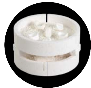
6 Stack sintering of restorations.
