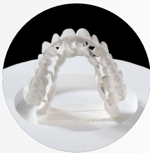
4 Separated and reworked restoration with sintering support.
