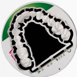
1 Bridges with skeletonized sinter support following the milling process.
