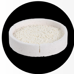
3 Fill the sintering dish MS with sintering pearls (a pearl bed of at least three layers).
