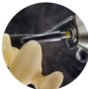
2 Processing with turbines under water cooling.
