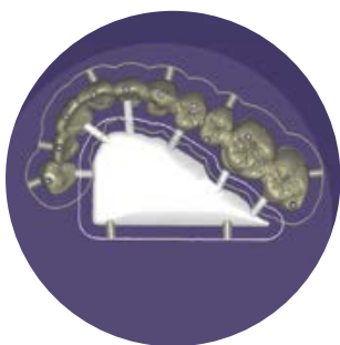
Sintering tongue and sintering drops.
