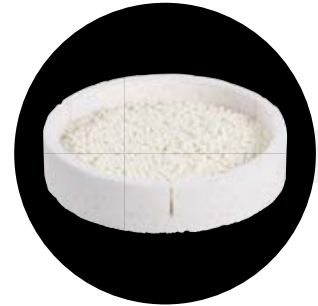
3 Fill the sintering dish MS with sintering pearls (a pearl bed of at least three layers).
