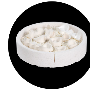
5 Sintering dish MS filled with restorations.
