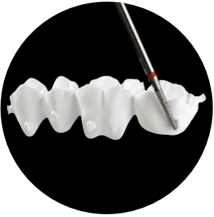
3 Grind connectors with diamond or carbide burr.
