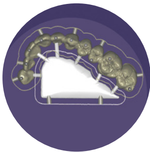
Sintering tongue and sintering drops.
