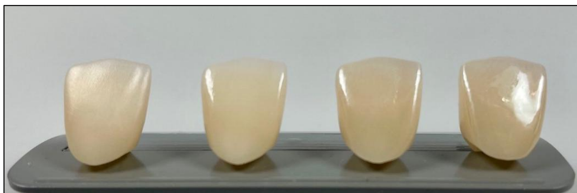
Figure 10: left to right AM-processed only, glazed, brushed with polishing paste and polished
