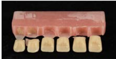
Figure 14 c: Fracture pattern; tooth base was only conditioned by sandblasting
