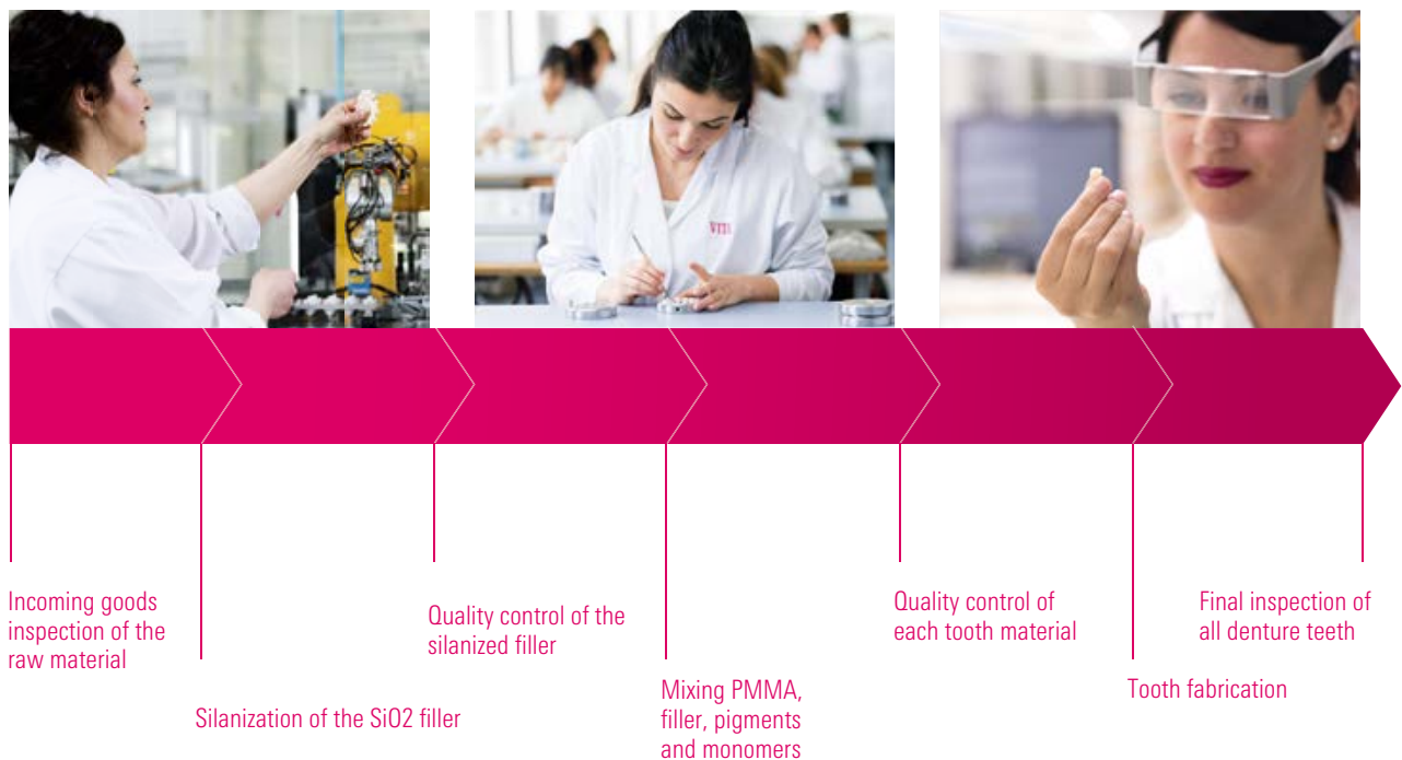
Figure 8: Manufacturing process of VITA denture teeth; source VITA R&D
