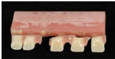
Figure 14 a: Fracture pattern; tooth base was sandblasted and coated with bonding agent
