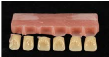
Figure 14 b: Fracture pattern; no surface treatment of the tooth base was performed
