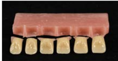
Figure 14 d: Fracture pattern; tooth base was only coated with bonding agent
