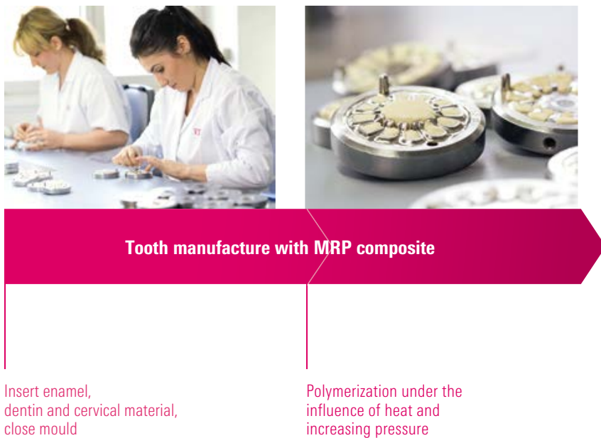
Figure 10 a: Schematic representation of the manufacturing procedure of denture teeth made from MRP composite; source VITA R&D
