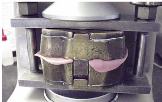
Fig. 23: ... the rest of the denture base is packed
