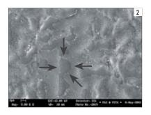
Fig. 1: SEM image of the etched surface of VITADUR ALPHA (magnification 5000 x).
