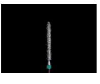
Chamfer diamond approx. 70-80  $\mu m$  for coarse preparation approx. 30  $\mu m$  for fine preparation
