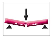
and hence in microcrack and crack formation which will finally lead to total fracture
