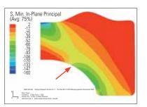
No notch stress thanks to convex preparation types and avoidance of box-shaped preparation
