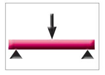
results in tensile stress in the ceramic (on the opposite side)
