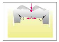
Box-shaped preparation results in tensile stress at the side opposite the one where the force is generated
