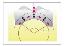
Convex cavity bottom design leads to the formation of compressive stress
