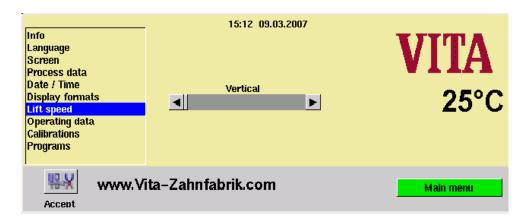
Adjust the lift speed with the slide control.
