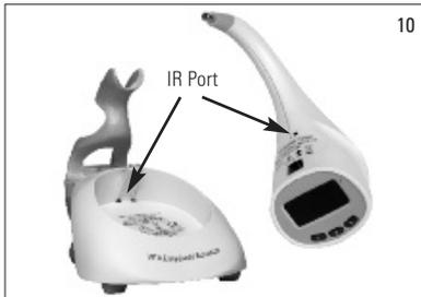
**⚠ Note:** Make sure not to block the IR ports above the labels located on the hand piece and the base unit (see IR ports, fig.10).
