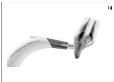
The probe tip must be placed perpendicular and flush to the tooth surface as shown in the adjacent figure (fig. 14).
