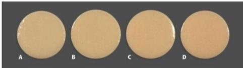
Fig. 2 Clear differences in terms of shade due to different pre-drying times with the same ceramic material: A: Without pre-drying, B: 2 minutes, C: 4 minutes, D: 6 minutes.
