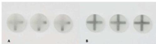
Fig. 3 Effect on transparency and shade effect when a crystal-clear material is not fully fired as a result of different lift positions (A: Furnace 25 % closed, B: Furnace 75 % closed)
