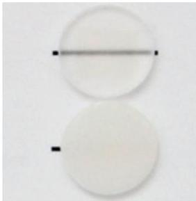
Fig. 6 Influence of the vacuum on the restoration; with a vacuum (see above), without a vacuum (see below).
