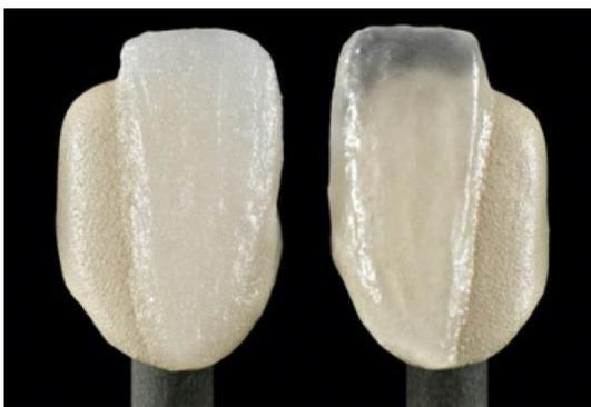
Fig. 8 Comparison of an incorrectly fired (left: underfired, poor vacuum) and a perfectly fired crown (right) with VITA VM 13 Window material.
