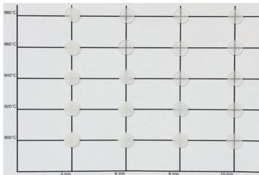
Fig. 4 Ceramic samples (Window material) with different degrees of firing depending on the heating time (x-axis) and temperature (y-axis)
