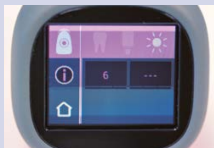
Fig. 5 Display of the Bleached Index according to the VITA Bleachedguide 3D-MASTER in the context of a professional tooth lightening.
