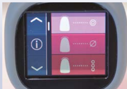
Fig. 1 Main menu of the OLED color touch display. Shown here: Basic shade measurement, average measurement and tooth area measurement.
