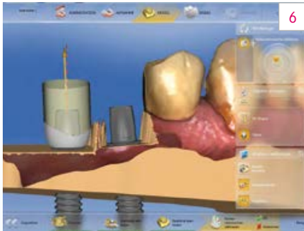
Fig. 6 Determination of the restoration axis for the computer-supported design of the abutment crowns.
