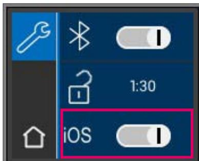
To communicate with iOS devices: Switch on Bluetooth® (I), switch to iOS (slide the iOS switch to the right (I)).
