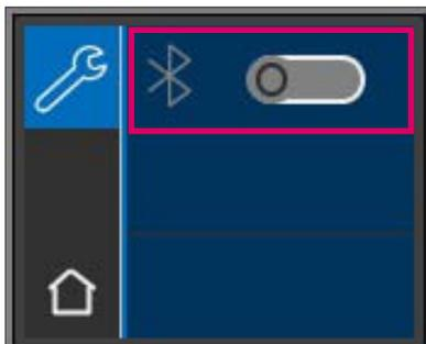
Bluetooth® indicator: Bluetooth® is switched off (0), slide the switch to the right to turn on (I)
